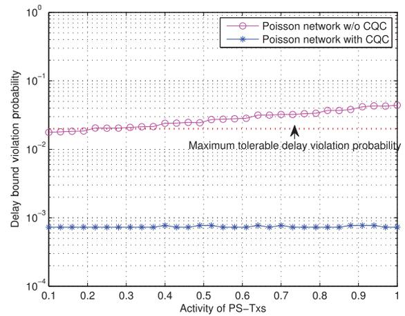
Fig. 4. Diversity mode for CQC with different activities of PS-Txs in large multihop CM2MN.
