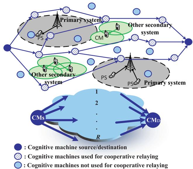
Fig. 1. Network model for network coded multipath routing algorithms in large multihop CM2MN.
