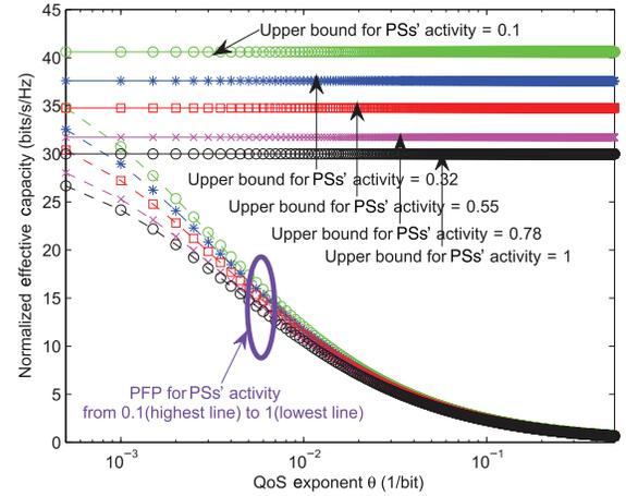
Fig. 2. Effective capacity with PFP and the upper bound with different activities of PS-Txs in large multihop CM2MN.
