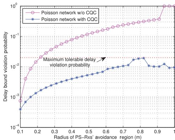
Fig. 5. Diversity mode for CQC with different radiuses of PS-Rxs' avoidance region in large multihop CM2MN.
