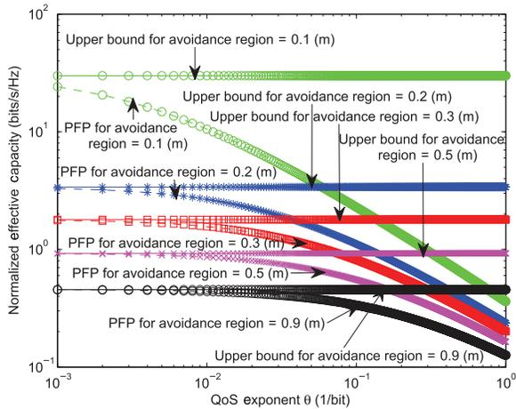
Fig. 3. Effective capacity with PFP and the upper bound with different radiuses of PS-Rxs' avoidance region in large multihop CM2MN.
